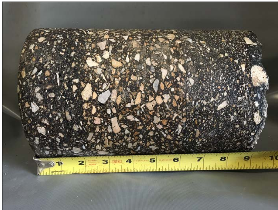
ASPHALT CORE AC-6
