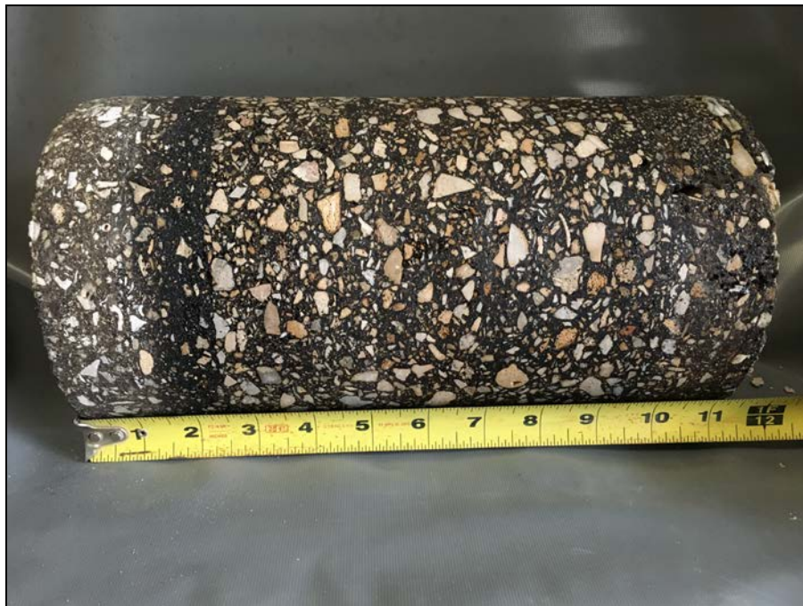
ASPHALT CORE AC-8
